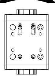
$M_z$  (static) = 131 in-lbs, 15 Nm.  $M_z$  (dynamic) = 162 in-lbs, 18 Nm.
