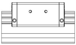
M<sub>y</sub> (static) = 28 in-lbs, 3.3 Nm. M<sub>y</sub> (dynamic) = 35 in-lbs, 4 Nm.
