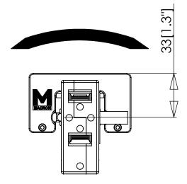
M<sub>x</sub> (static) = 19 in-lbs, 2 Nm. M<sub>x</sub> (dynamic) = 23 in-lbs, 2.5 Nm.
